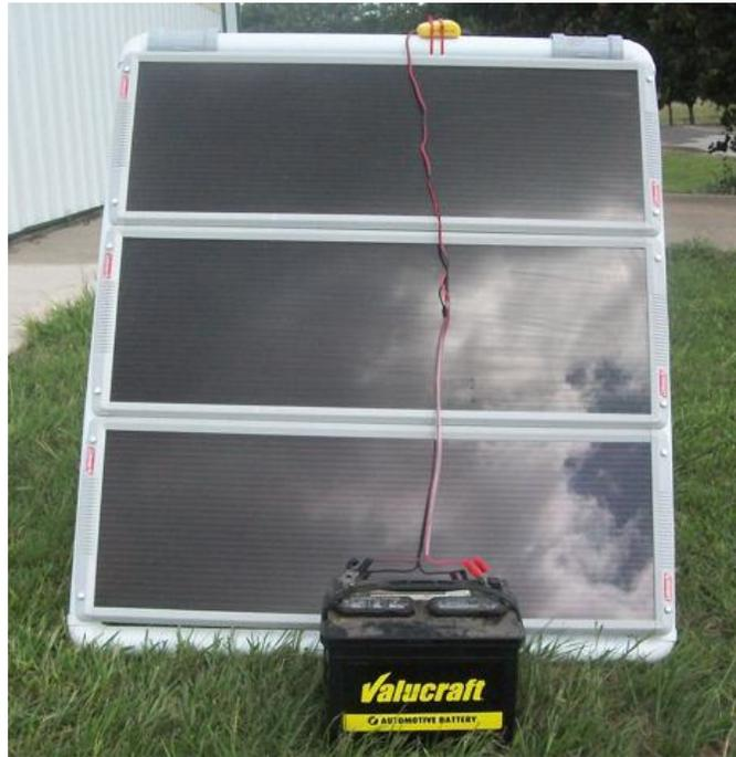
We bought three 15-watt solar panels from Harbor Freight\*, a tool store. They come with a PVC stand, a yellow charge controller, and some clamps to connect them to a 12-volt battery. You can use the battery with an inverter to produce some electricity for use at night if your home's electrical power is off.
