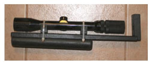
The problem with using a rifle scope as a telescope is that everything gets out of focus when you put the rifle scope up to your eye. When a rifle scope is mounted on a rifle, there is space (called "relief") between the scope and your eye. (Rifle recoil would get your eye, if there were no relief. What a relief relief is!)
